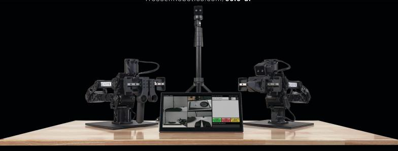
The Solo AI is a portable desktop machine learning data collection lab, consisting of a leader-follower arm pair, a portable touchscreen with GUI, two Intel RealSense D405 RGB depth cameras, and optional compute solutions. It makes data collection in the field a breeze with it's simple setup and tear-down, and intuitive data collection touchscreen app.
